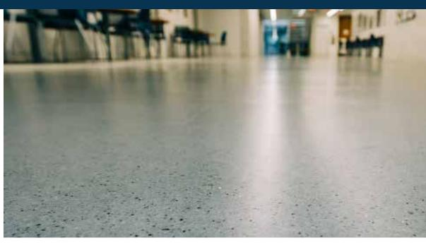
Stoncrete EFX is a troweled, epoxy mortar system that has the look and feel of polished concrete, but with longer lasting durability and performance. Developed for commercial spaces like school corridors, office spaces and retail stores, it is also well-suited to industrial facility lobbies and corridors. Stoncrete EFX can be used for new flooring or to resurface an existing floor.
